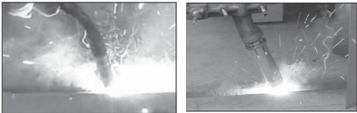
(b) “J-STAR® Welding”; KC-550,DCEN(Direct current electrode negative), Welding current:380A
